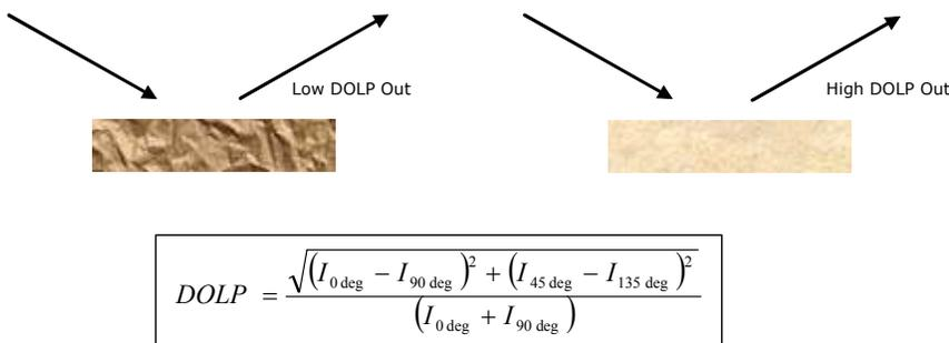
Figure 5 -Degree of Linear Polarization by Reflection (Scatter)
