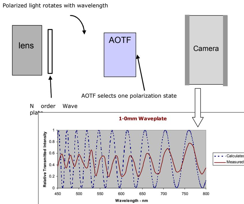
Figure 7 -Schematic of Spectral-Polarimetric Imager Using A Single Multi-Order Wave plate.
