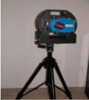
Figure 6 -AOTF HSI camera. Mechanical rotation about an axis along the optical centre of the objective lens allows capture of images polarized at 0°, 45°, 90° & 135°
