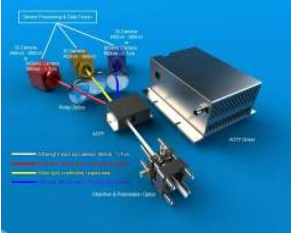
**Figure 5 - Three Camera HSI Unit Exploiting AOTF operating in Dual- Polarization Mode**
