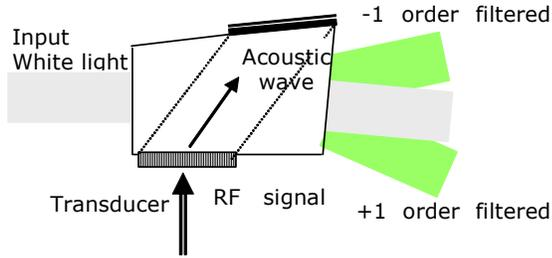
Figure 2 - AOTF with Dual Output
