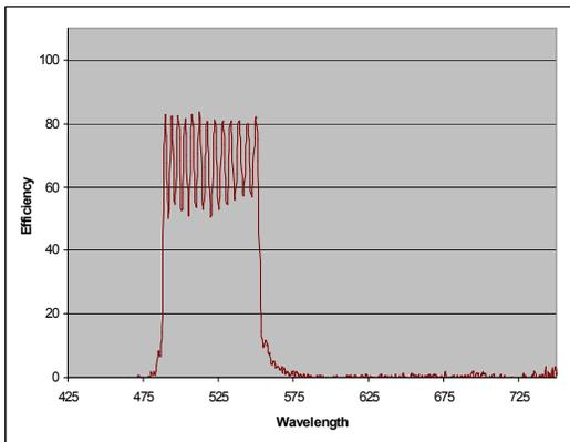
Figure 1 - AOTF Driven With Multiple (13) Frequencies
