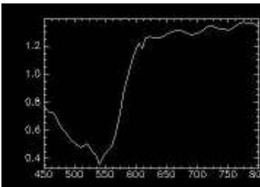
Figure 11 - Reflectance spectrum of artificial soiling.
